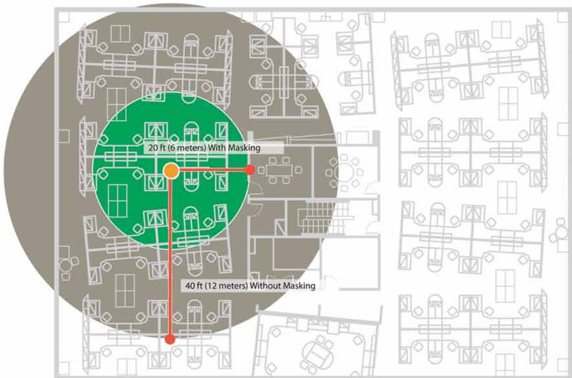
Diagram 5: Sound Masking's Effect on Intelligibility
